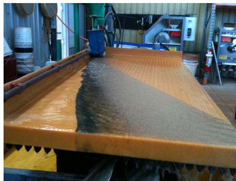
Hemerdon ore on a shaking table showing black Wolframite concentrating
